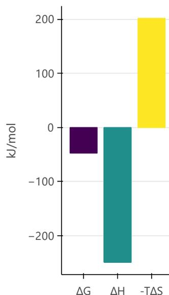
$$\Delta H = \text{slope} \cdot R = -30096 \text{ K} \cdot 8.314 \frac{\text{J}}{\text{mol} \cdot \text{K}} = -250.2 \frac{\text{kJ}}{\text{mol}} = -59.8 \frac{\text{kcal}}{\text{mol}}$$
