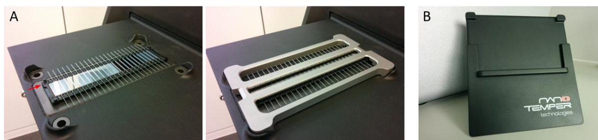
Figure 4: Manual sample loading for the Prometheus NT.Plex. (A) When placed correctly, the plastic chip structure frames the thermal element and the capillaries rest on top of the thermal element. The metal lid is then placed slowly and evenly inside of the guiding structures, with the rubber padding securing the capillaries in place. The red arrow indicates the imprinted number ① on the capillary chip. (B) The Capillary Chip Filling Station is recommended for manual loading of capillary chips from microtiter plates.
