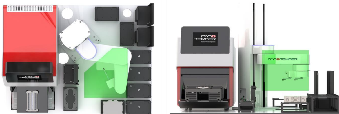
Figure 4: The robotic arm's safe zone is indicated in green. The robotic arm is safe when its wrist is in the safe zone. As a rule of thumb, manually move the robotic arm's gripper so that the gripper fingers are located above the waste.
