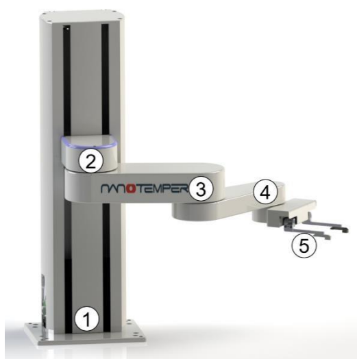
Figure 3: The robotic arm anatomy and joints. (1) z column, (2) shoulder, (3) elbow, (4) wrist and (5) gripper and gripper fingers.
