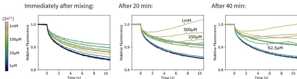
$\text{Zn}^{2+}$ -induced aggregation of tau for  $\text{Zn}^{2+}$  concentrations  $> 50 \mu\text{M}$  after a lag time of 20–40 minutes.
