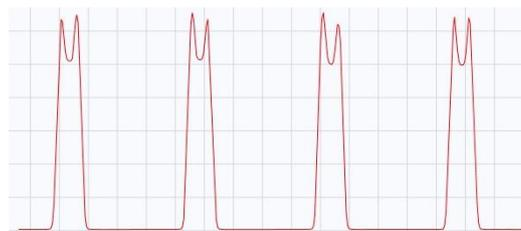
**Fig. 3** Capillary scan after the measurement in standard treated capillaries: the double peaks clearly indicate unspecific binding of labeled Hsp90 to the capillary walls.
