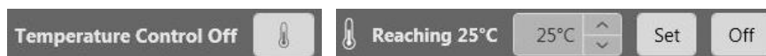
Figure 5: Temperature controls. Left panel: click the thermometer icon to open the temperature control. Right panel: choose the desired temperature using the arrow buttons, then click Set to start the temperature control.
