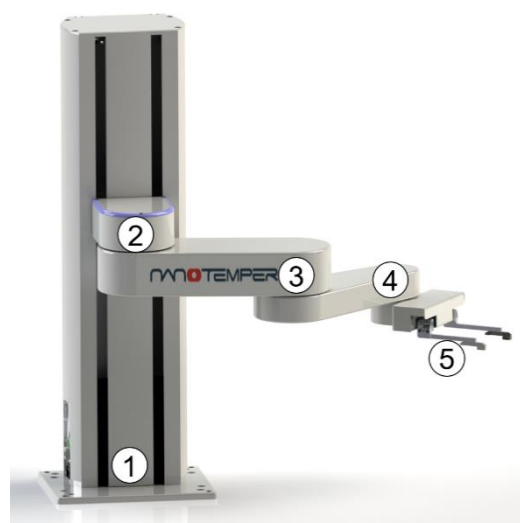
Figure 4: The robotic arm anatomy and joints. (1) z column, (2) shoulder, (3) elbow, (4) wrist and (5) gripper and gripper fingers.
