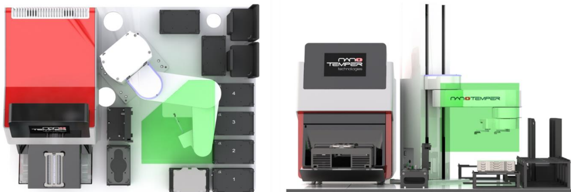
Figure 5: The robotic arm's safe zone is indicated in green. The robotic arm is safe when its wrist is in the safe zone. As a rule of thumb, manually move the robotic arm's gripper so that the gripper fingers are located above the waste.
